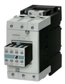
CONTACTOR, AC-3 45 KW/400 V, DC 24 V, 2 NO + 2 NC, 3-POLE, SIZE S3, SCREW CONNECTION
